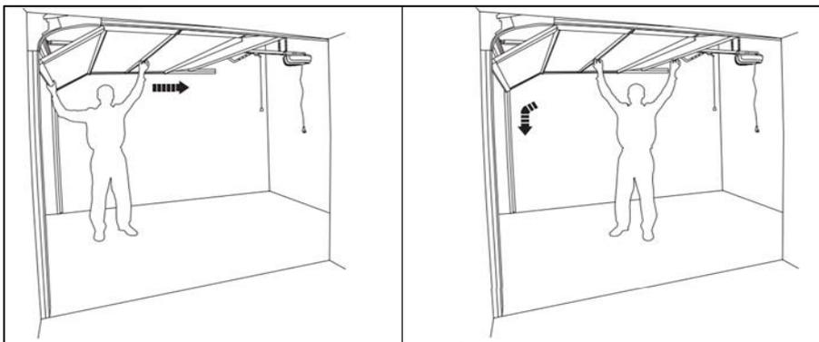
**Two Stage Trolley- Manual Release Mechanism**
